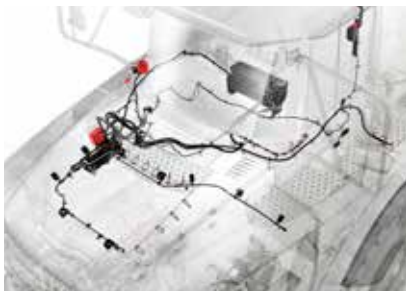
Volvo fire suppression system
